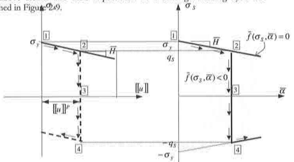
Figure 2-9– Elasto-plastic discrete model: loading-unloading cycle
