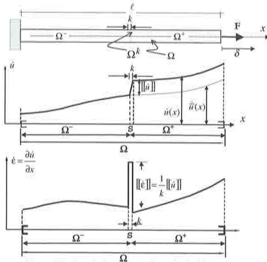
Figure 2-7– Regularized strong discontinuity kinematics
