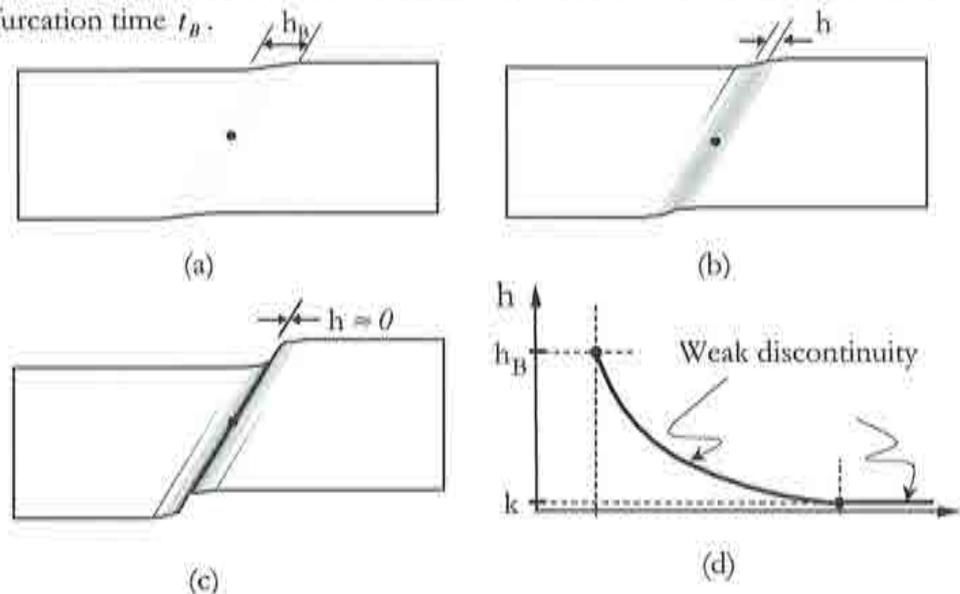
Figure 4-1– Mechanism of formation of a strong discontinuity: (a) Discontinuous bifurcation into a weak discontinuity. (b)-(c) Collapse into a strong discontinuity of null bandwidth.
