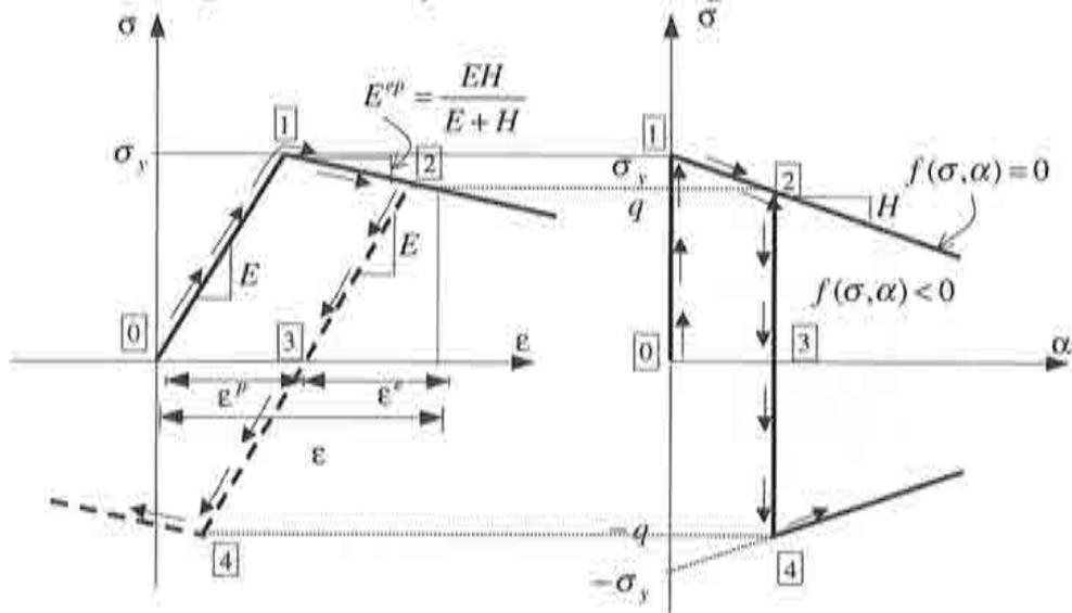
Figure 2-2—Elasto-plastic model: loading-unloading cycle
