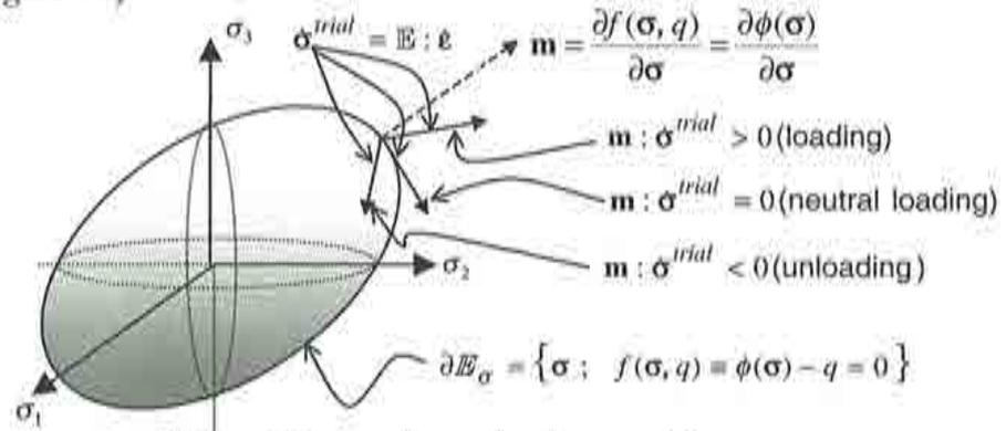
Figure 4-2– Loading-unloading conditions
