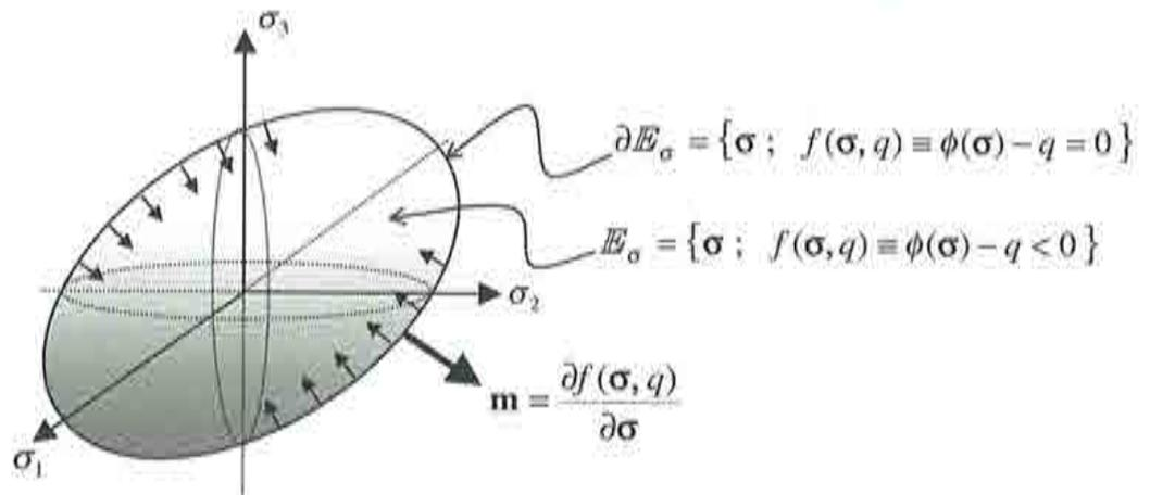
Figure 3-5– Elasto-plastic 3D model: yield surface and elastic domain in the stress space
