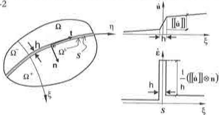
Figure 3-2– Regularized strong discontinuity kinematics
