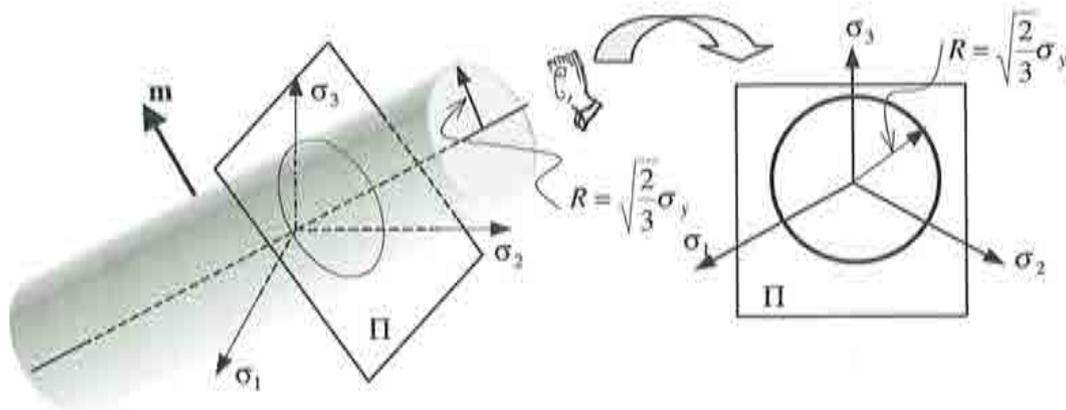
Figure 4-10- J<sub>2</sub> (von Mises) plasticity model
