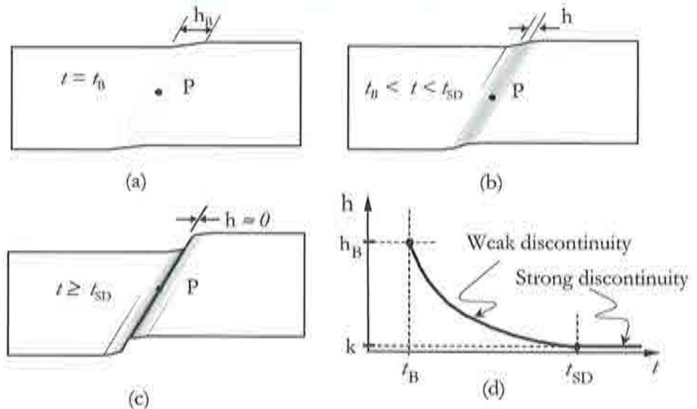
Figure 3-3— (a) to (c): mechanism of formation of a strong discontinuity. (d) variable bandwidth model
