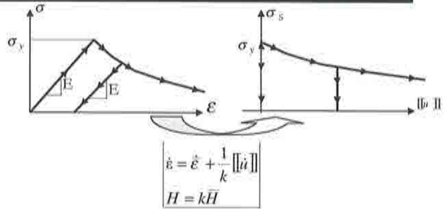
Figure 2-10– Original continuum and induced discrete elasto-plastic models
