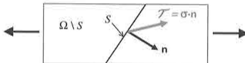
Figure 3-6– Traction continuity across the discontinuous interface
