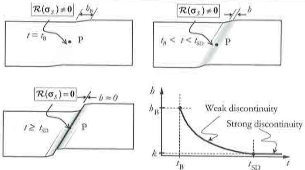
Figure 3-8- The strong discontinuity conditions and the variable bandwidth model
