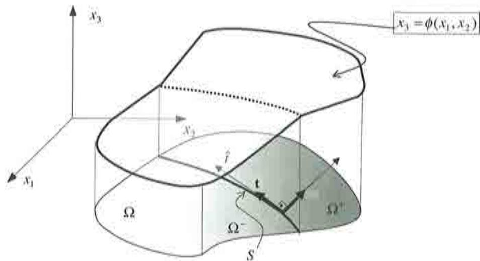
Figure 1-6— Continuous scalar field with discontinuous gradients
