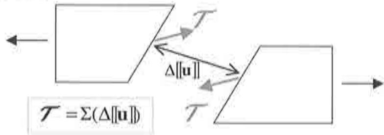
Figure 3-10– Discrete constitutive model at the discontinuity interface
