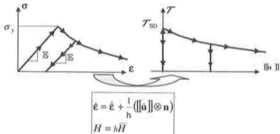
Figure 3-11– Original continuum and induced discrete elasto-plastic models
