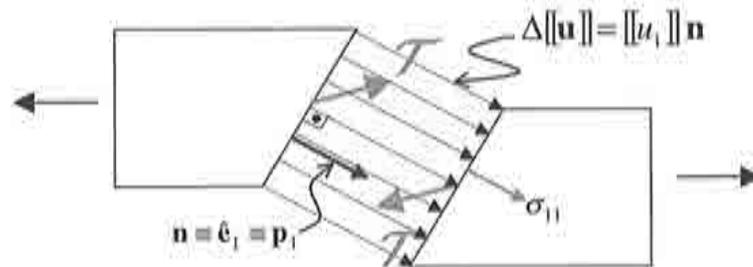
Figure 3-13– Mode I of fracture
