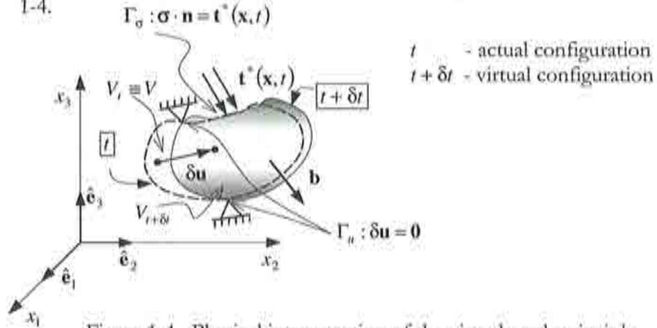
Figure 1-4— Physical interpretation of the virtual work principle
