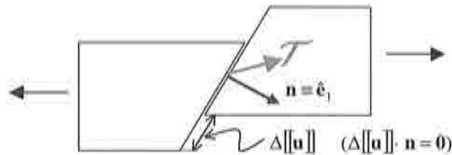
Figure 3-15– Mode II of fracture
