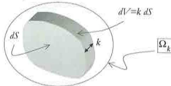
Figure 2-8– Differential of volume at the discontinuity interface
