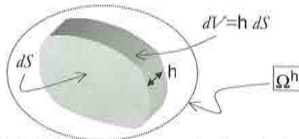
Figure 3-9– Differential of volume at the discontinuity interface
