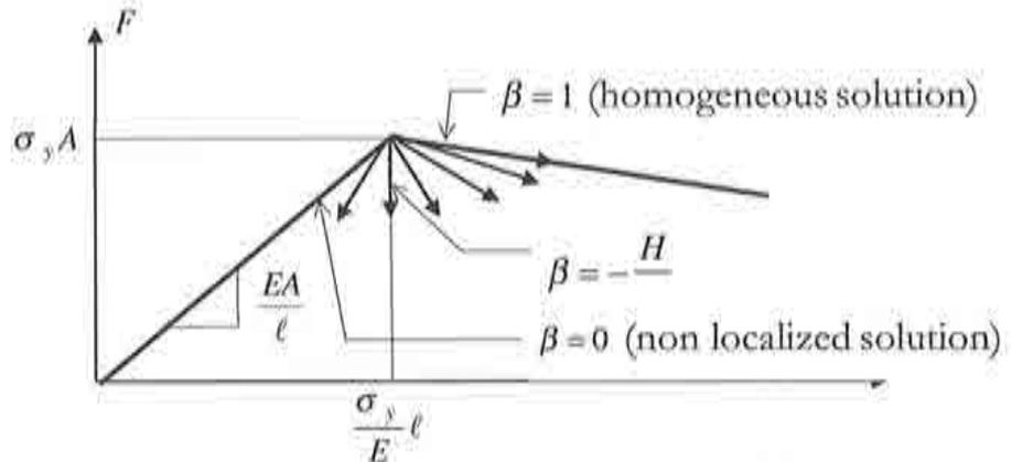
Figure 2-4— Solution of the 1D localization problem
