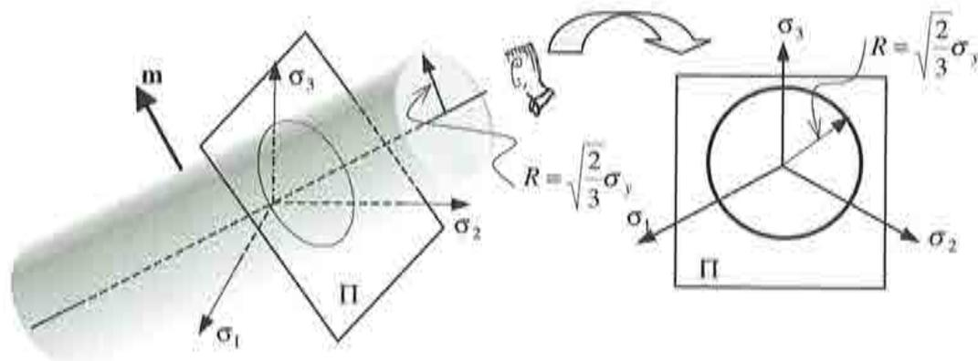
Figure 3-14—J<sub>2</sub> (von Mises) plasticity model
