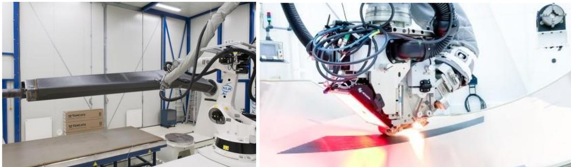
**Figure 3:** Fibre placement technology which is used for the manufacturing of the skin. [6, 7]
