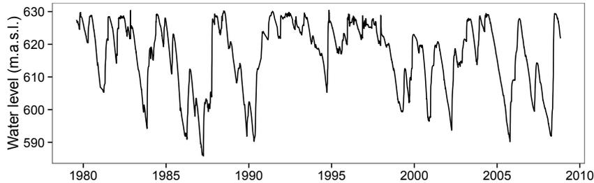
Figure 2: Time series of the reservoir level at La Baells Dam.
