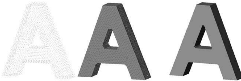
Figure 12. Three-dimensional arbitrary geometry. Left: boundary nodes from the point distribution generated by GID with constant h and 8,452 nodes. Center: boundary surface for 8,452 nodes. Right: boundary surface for 106,947 nodes
