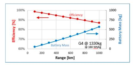
**Figure 2.** Adding battery weight decreases efficiency, which was revealed by an internal analysis based on G4 Vehicles (Golf class). Reproduced from [10].
