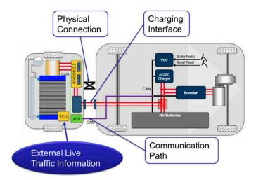
Figure 4. Intelligent FC range extender demonstration.
