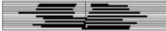
Figure 5. Approximated localisation of delamination from experimental results by Hou et al. (2000). The figure represents a through-thickness view of a quarter of the target laminate. Middle vertical line indicates the corner.
