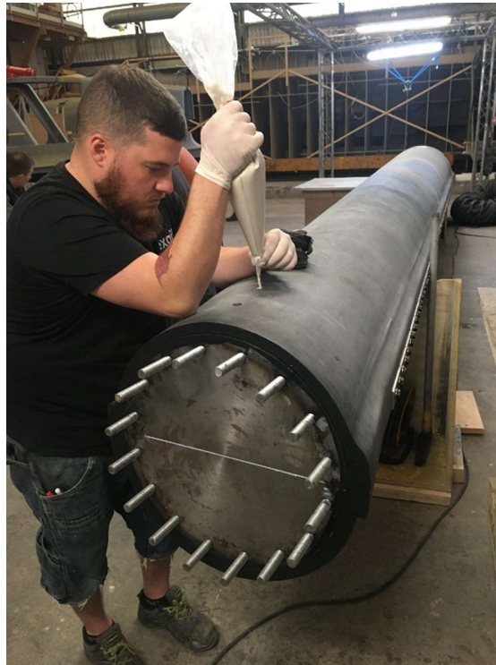
Figure 31 : resin casting for top ring
