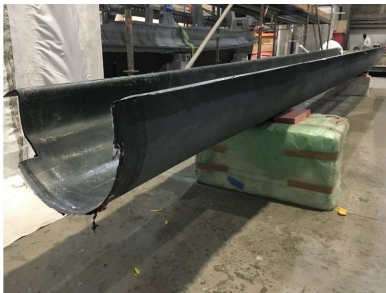
Figure 19 : half mast unmoulded
