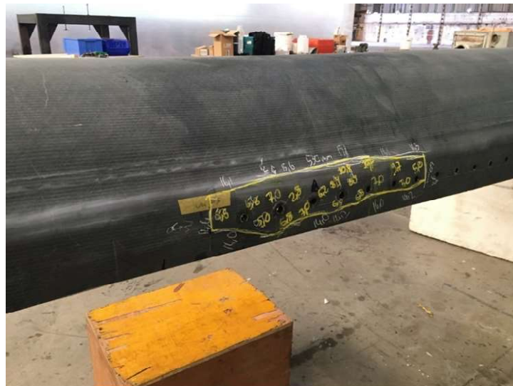
Figure 26 : results of ultrasonic NDT
