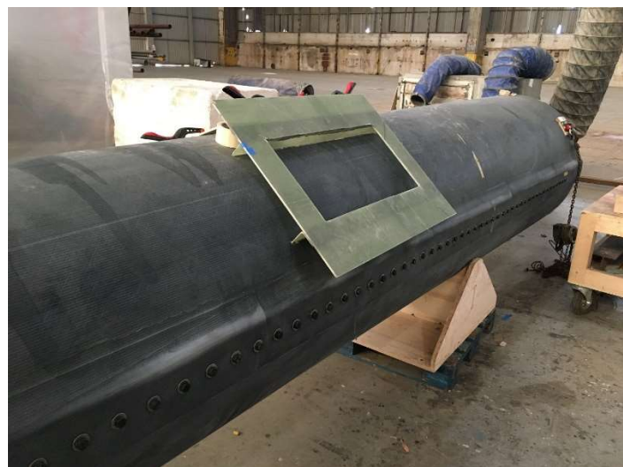
Figure 34 : electrical box support laminated
