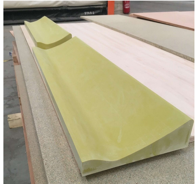
Figure 11 : section of plug finished
