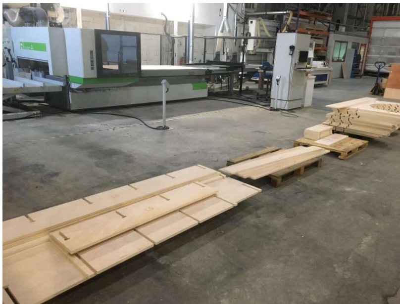
Figure 9 : panels cut by CNC
