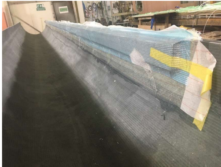
Figure 20 : lamination of the steel insert
