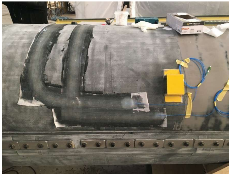
Figure 37 : optic fibre laminated to the tower
