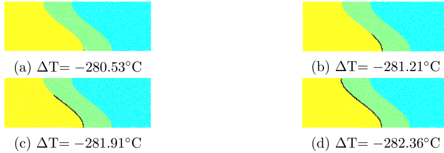
Figure 10: TGO/BC interface delamination as function of thermal loading (unit cell)
