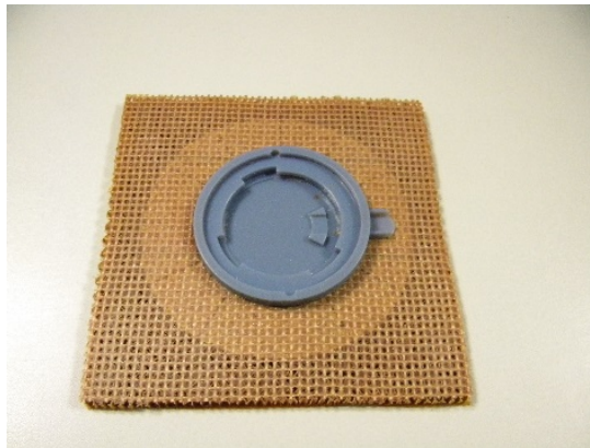
Figure 5: Test sample after curing with a bonded insert
