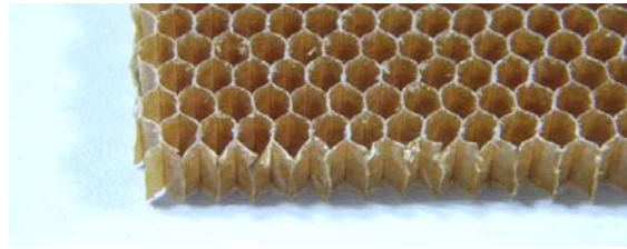
Figure 3: paper honeycomb. 6,5mm thickness. Can be used as a sandwich core, healthy or crushed
