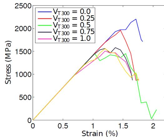
**Figure 1.** Stress-strain diagrams for AS4-T300 hybrid composites with various hybrid.
