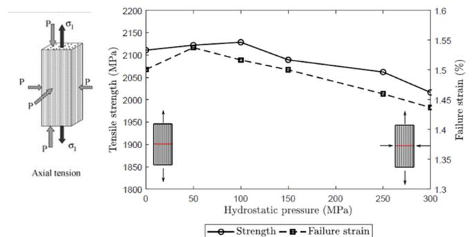
**Figure 2.** Strength and failure strain as a function of the applied hydrostatic pressure.
