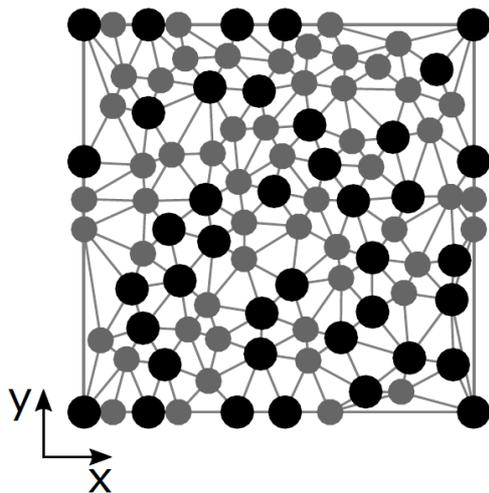
**Figure 3.** 2D mesh for a periodic RVE with a random fibre distribution.
