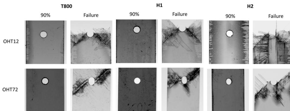
**Figure 6.** X-ray images of the open-hole tension specimens: 12 mm and 72 mm wide.
