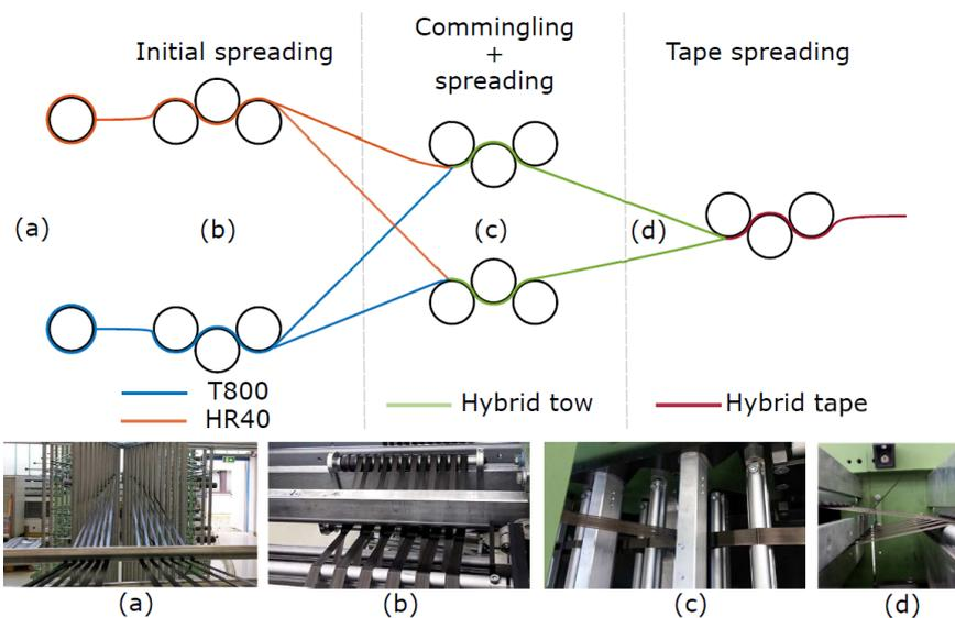
**Figure 7** Schematic representation of the spreading process for hybrid materials.
