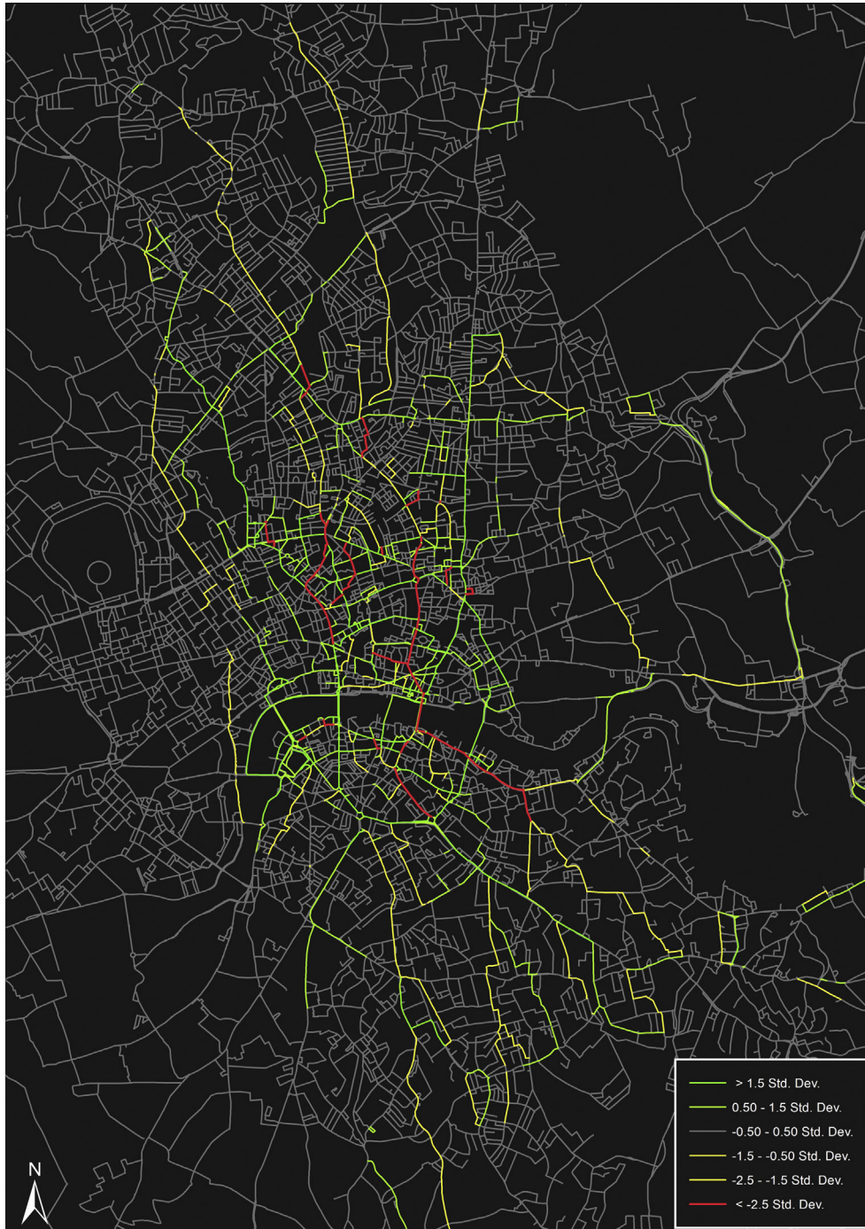
Fig. 4. Standard deviations around differences between observed traffic flows and alternatives calculated using an optimal distance metric between North and South-East postcodes.
