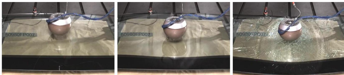
(c) Initial fracture of test number 7 between 8 and 9 ms.
