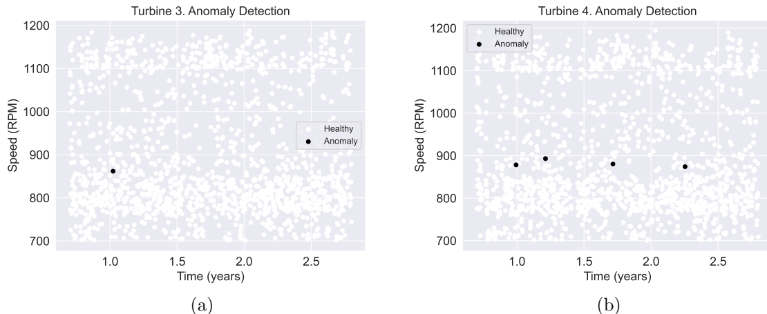
Figure 6: Testing data with detected anomalies (false alarms) in Turbines 3 (a) and 4 (b).
