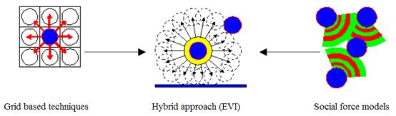
Fig. 1: Space modelling techniques (D. Vassalos et al., 2003)
