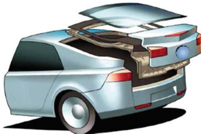
Figure 75 – Application of dismantlable adhesives containing thermally expandable microcapsules in the automotive industry (ECODISM project)
