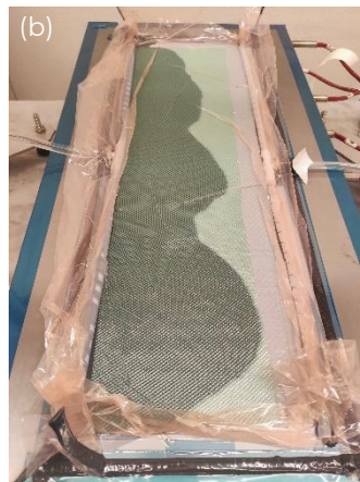
Figure 296 – Infusion process: (a) Before infusion; (b) During infusion; (c) After infusion
