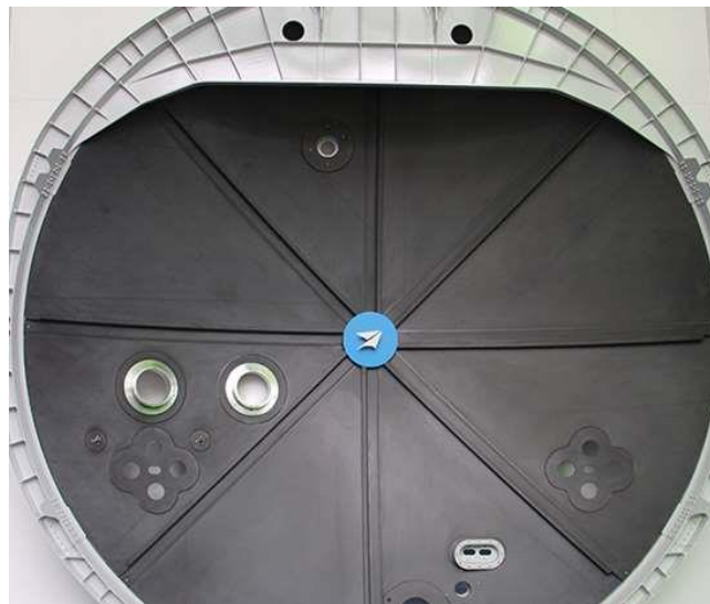
Figure 107 – 1:1 demonstrator of a thermoplastic carbon fibre-reinforced plastic (CFRP) welded pressure bulkhead for a single-aisle jetliner
