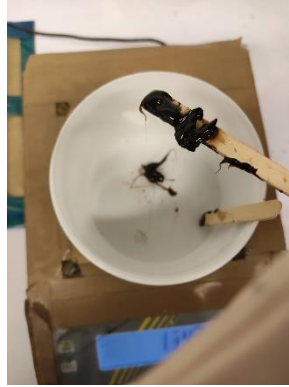
Figure 306 – Epoxy (Component A) becoming solidified after a few minutes at T_{amb} .
