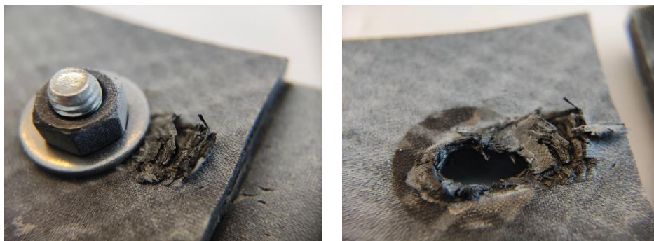
Figure 322 – Specimens' failure surfaces – bearing failure
