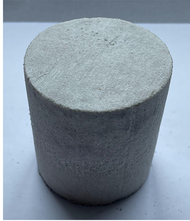
Figure 3: Clayey-silt hydrate sediment sample
