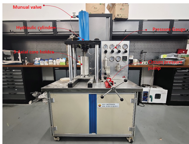
Figure 2: Platform of the triaxial seepage experimental device for hydrates
