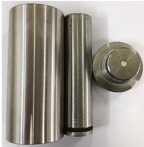
Figure 1: Hydrate sediment preparation kettle
