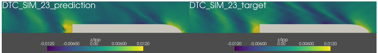
Figure 5: Iso-surface of water volume fraction = 0.5 colored by the non-dimensional free surface elevation. L_{PP} is the length between perpendiculars. Left: DLP prediction. Right: CFD result.
