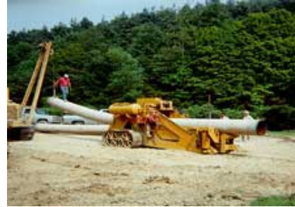
FIGURE 4.1-3 Pipe Bending Machine (Reproduced with permission.)
