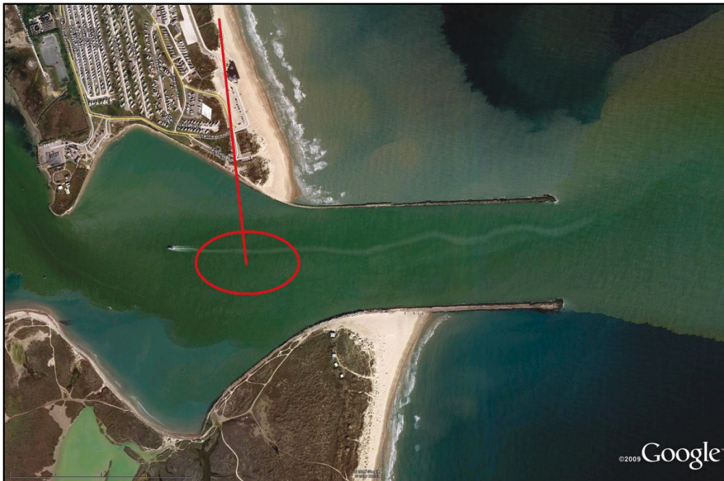
Figure 8-18. Schematic location of the dredging location for a dedicated pump plant and associated discharge pipe (from Google Earth https://www.google.com/earth/ ).
