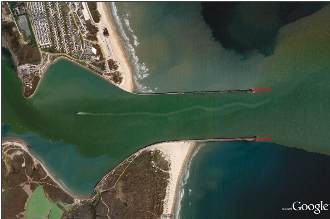
Figure 8-8. Brazos Santiago Inlet showing the Seaward Jetty Extension Alternative in red (from Google Earth https://www.google.com/earth/ ).
