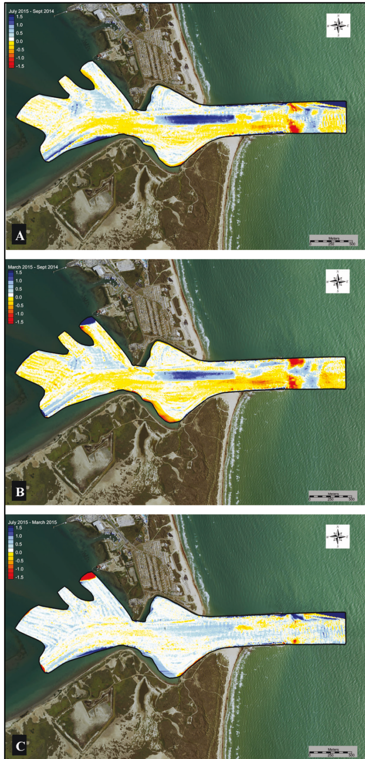
Figure 4-30. Bed change in meters. Positive values denote deposition. Negative values denote erosion. (A) September 2014 to July 2015, (B) September 2014 to March 2015, (C) March 2015 to July 2015 (from Google Earth https://www.google.com/earth/ ).
