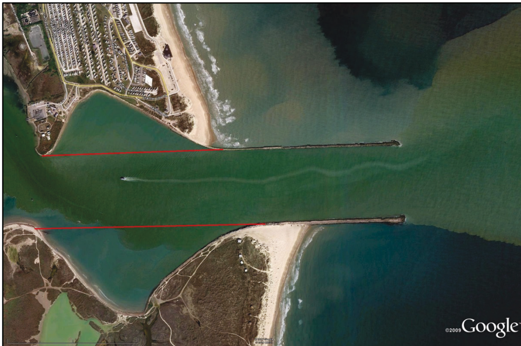
Figure 8-11. Brazos Santiago Inlet showing the Interior Jetty Straightening Alternative in red (from Google Earth https://www.google.com/earth/ ).
