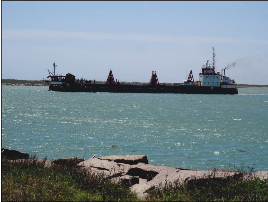
Figure 2-3. Hopper dredge Newport, dredging Brazos Santiago Inlet, 10 April 2014.
