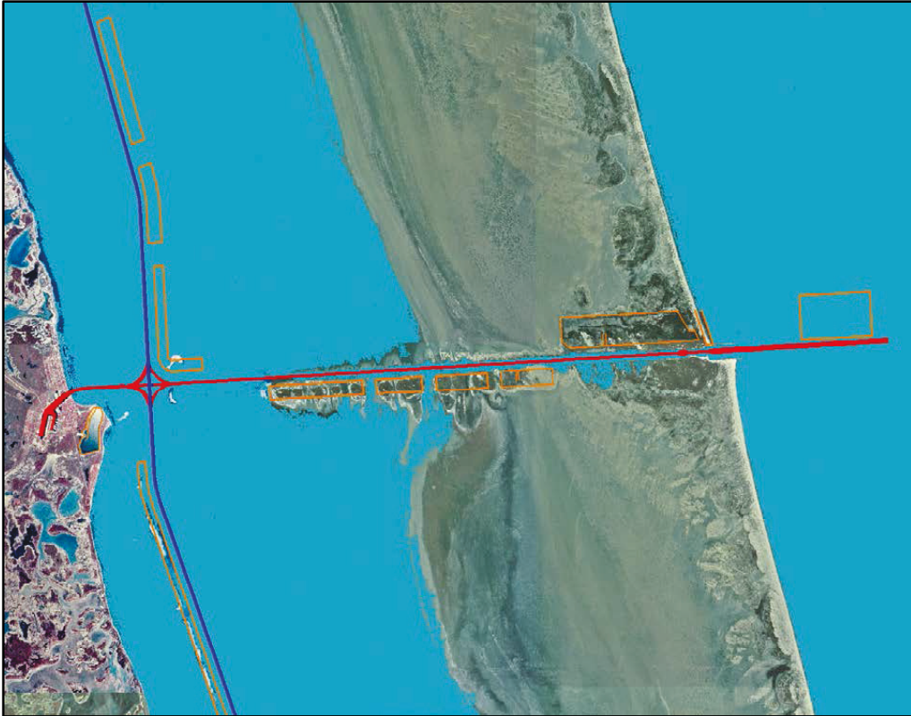
Figure 2-6. Mansfield Channel (red line); Gulf Intracoastal Waterway, GIWW (blue line); Designated dredge deposition areas (tan boxes) (after USACE [2014c]) (from Google Earth https://www.google.com/earth/ ).
