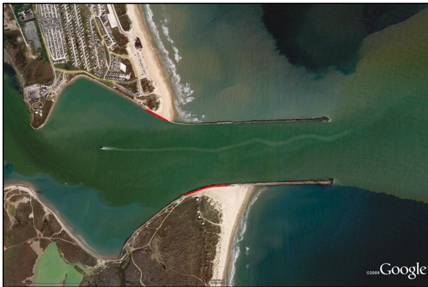
Figure 8-15. Brazos Santiago Inlet showing likely locations (in red) to increase the jetty height for the Heighten Jetty Alternative (from Google Earth https://www.google.com/earth/ ).
