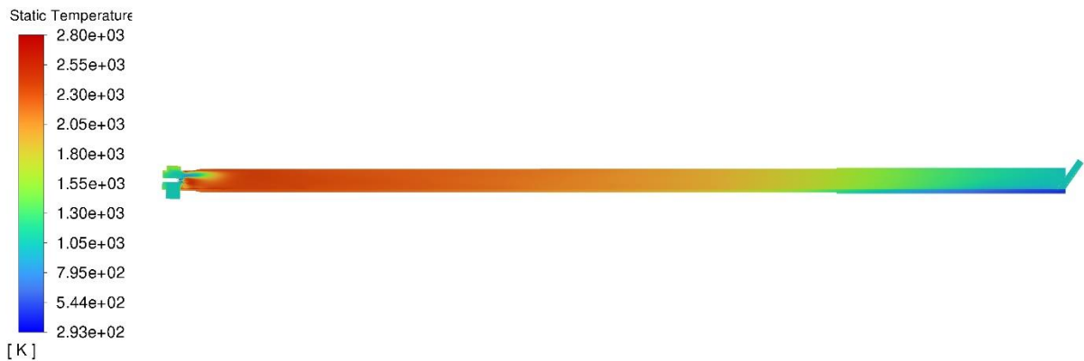
Figure 4: Flame temperature distribution after biomass injection, showing peak values near the burner (~2300–2500 K) and a gradual decrease toward the kiln outlet.
