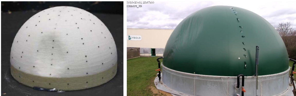
Figure 3: Model of the wind tunnel test [2, p. 10 Abb. 9], left; picture of the experimental set-up [KIT-fgb]
