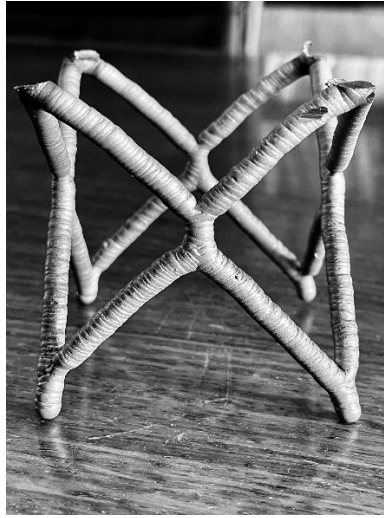
Figure 1: A specimen fabricated using the “dot-by-dot” WAAM process
