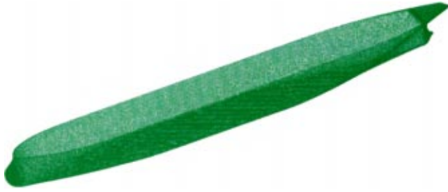
Fig. 8 KVLCC2 model. Surface mesh used in the analysis.
