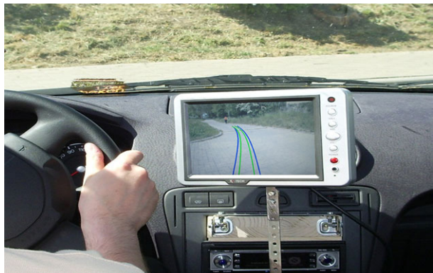
Fig. 10 The HMI of a Visual Assistance System to back up a trailer
