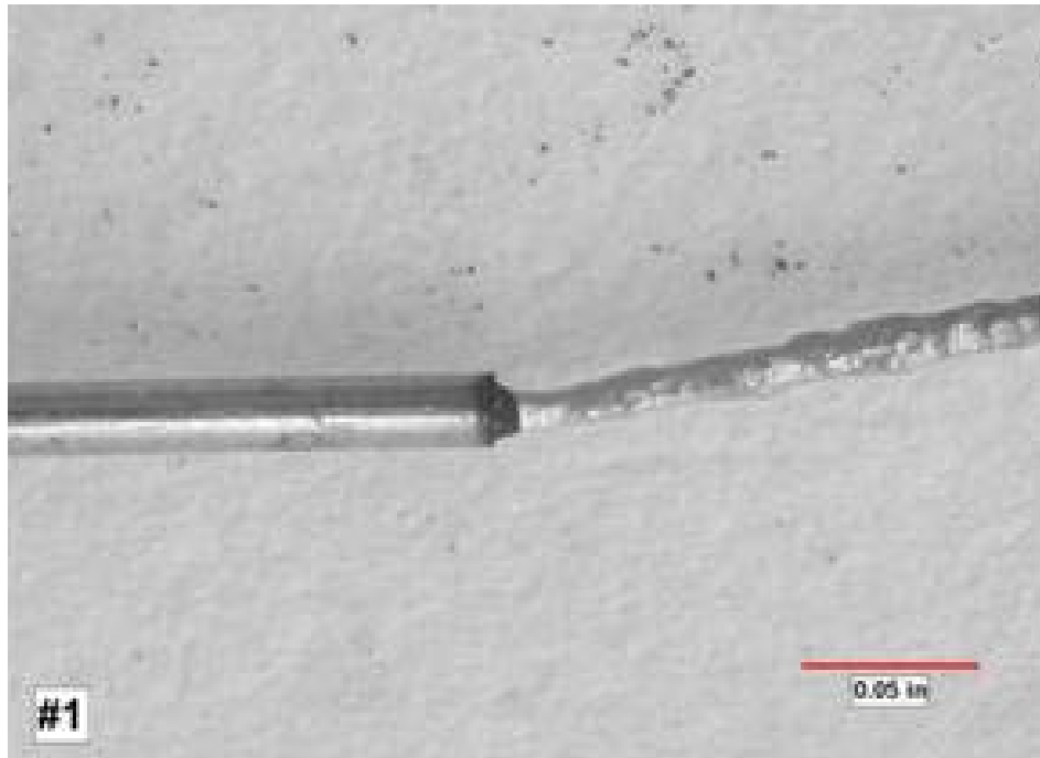
Figure 3-16. Post-test appearance of 0.5 mm steel wire used as ER probe after exposure to 0.1M NaCl for nearly 12 weeks.
