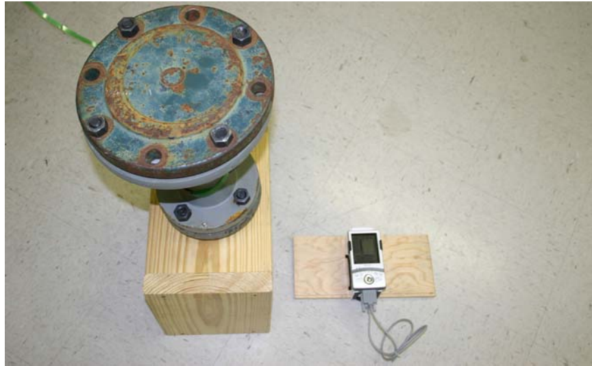
Figure 2-7. 6” pipe section with enclosed transmitter (left) used to ascertain UWB transmissibility to antennae receiver (right) within a sealed pipe.
