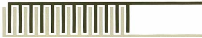
Figure 3-1. Planar view of thin film interdigitated galvanic couple sensor. This sensor is currently composed of conductive carbon (black lines) and silver laid out on Mylar.
