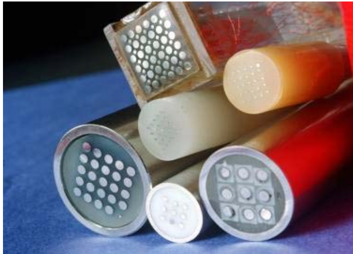
Figure 3-2. End view of several different versions of the SwRI developed MAS probe.
