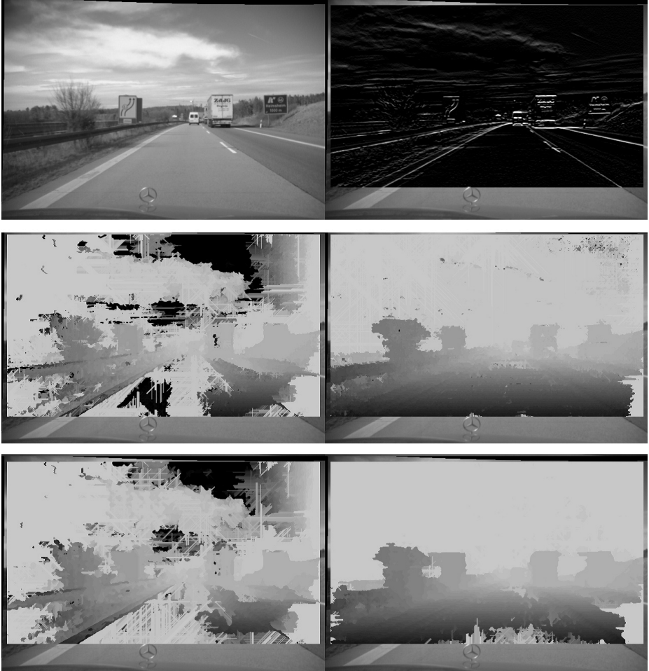
Fig. 4. Top: image of original input sequence (left) and its Sobel image (right). Middle: results of SGM (reference configuration) on original image pair (left) and on Sobel image pair (right). Bottom: results of SGM (using our optimized configuration f) on original image pair (left) and on Sobel image pair (right).
