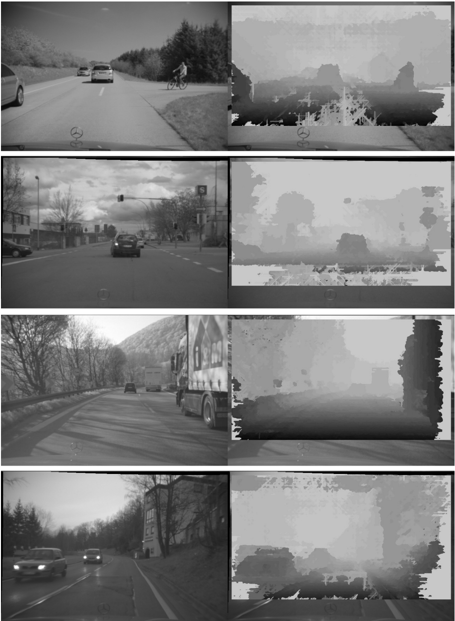
Fig. 5. Left: example of a right input image of the processed sequence. Right; depth maps, after Sobel preprocessing, and using SGM with the optimized configuration.
