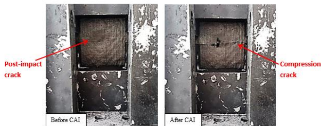
Figure 15. Cross-Ply 16 plies after 50 J impact before (left) and after (right) CAI
