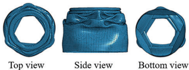
Figure 7: The compressive deformation mode
