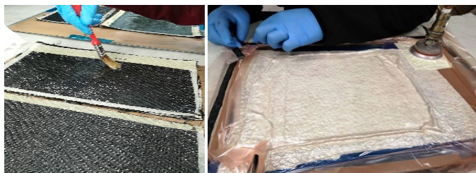
Figure 3. Fabric impregnation (left) and vacuum bagged materials before the autoclave processing (right).
