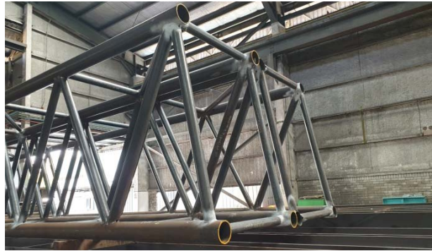
Figure 18: Main girder before galvanisation
