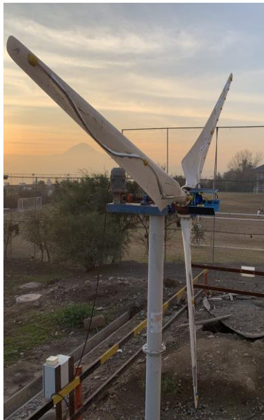
Figure 1: Experimental wind turbine mock-up
