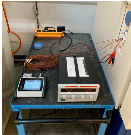
Figure 5: test setup: data logger (left) and power unit (right)
