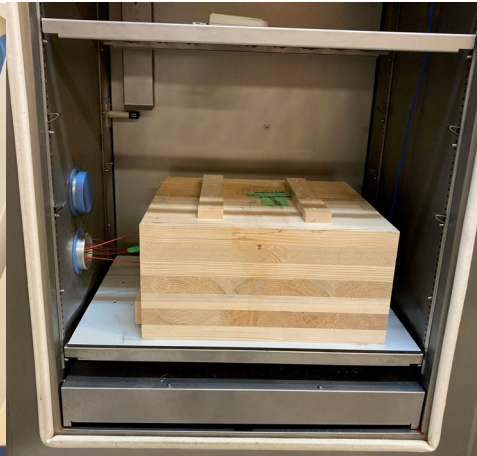
Figure 6: test setup: casted test specimen in the climate chamber
