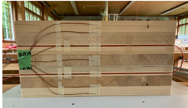
Figure 4: test setup: temperature sensors and heating wires before casting
