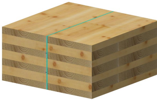
Figure 1: casted overall test specimen with two heating wires
