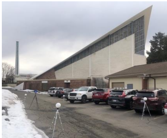
Figure 2: Laser scanning set-up and control points
