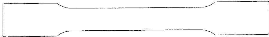
Figure 1. Specimen for material tension test
