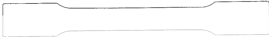
Figure 1. Specimen for material tension test
