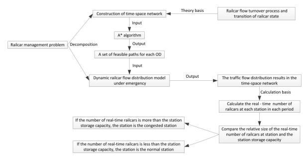
Figure 3. Flowchart of predicting traffic congestion in a station in an emergency.
