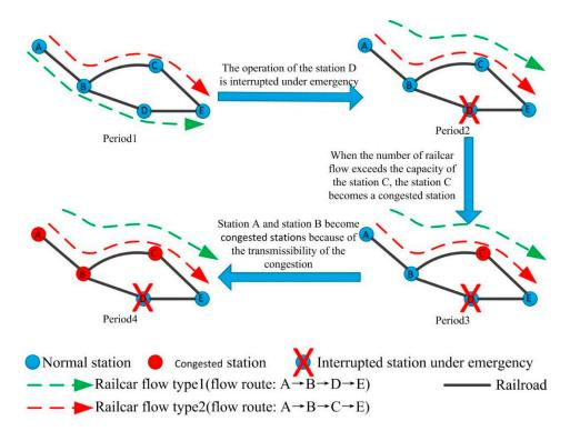
Figure 1. Schematic diagram of the process resulting in traffic congestion due to the emergency.
