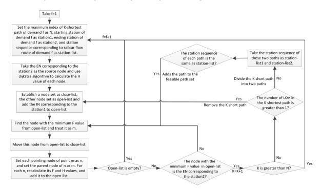
Figure 5. Flowchart of improved A\* algorithm.
