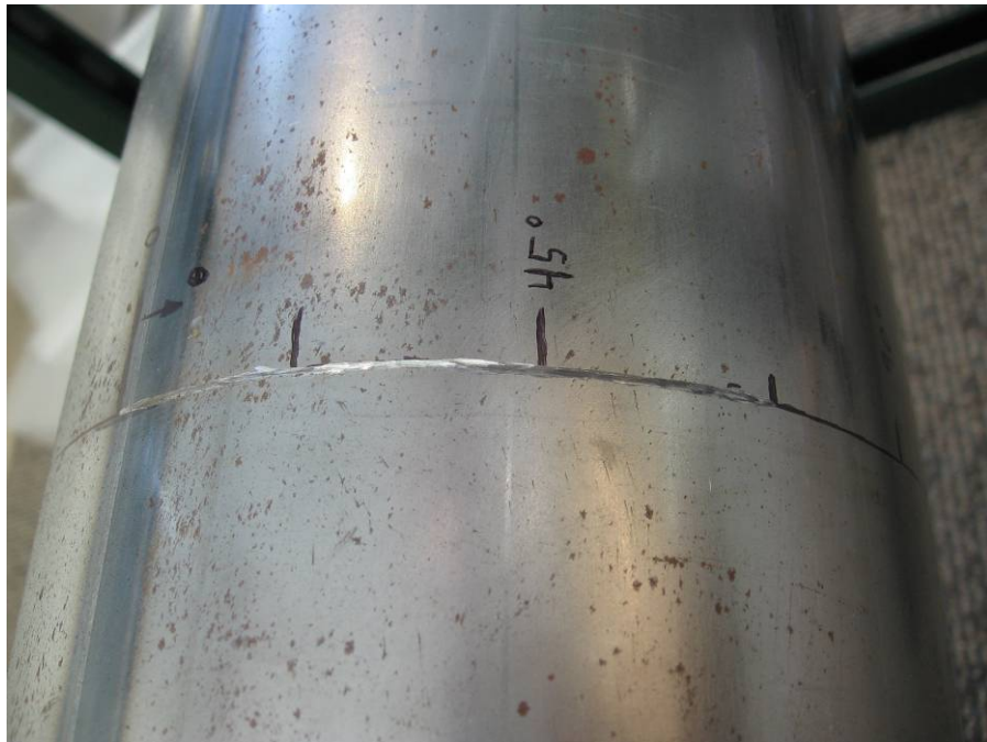
Figure 5.3: Circumferential notch, 50% through thickness, 0.0^\circ to 67.5^\circ
