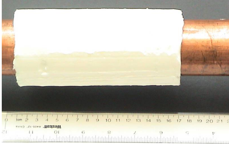
Figure 7.3: Layer of vegetable shortening for damage case 3
