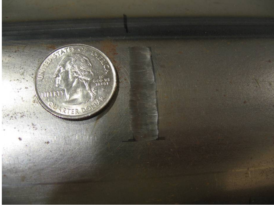
Figure 5.8: Surface grinding, 0.0° to 22.5° long, 0.25-in (6.4-mm) wide
