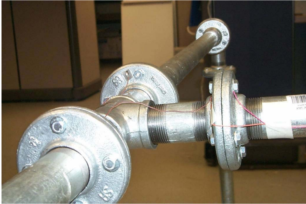
Figure 2.5: Application of impedance methods to a simple pipeline structure (Park, et al. 2001)
