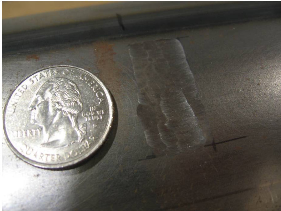
Figure 5.9: Surface grinding, 0.0° to 22.5° long, 0.50-in (12.7-mm) wide
