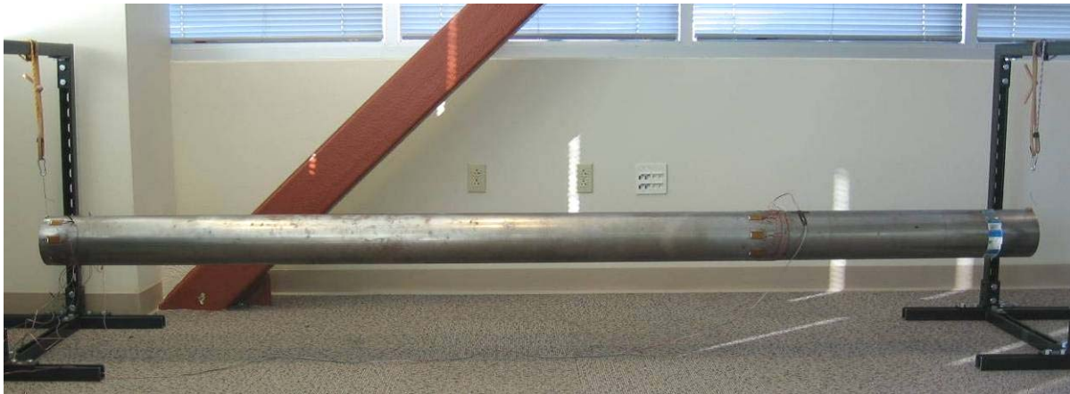
Figure 3.1: Apparatus for Lamb wave measurements
