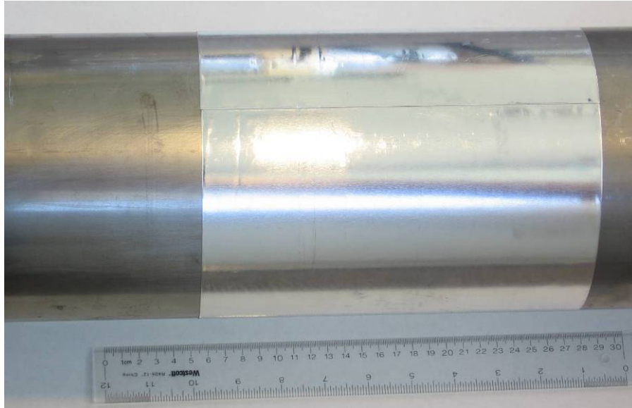
Figure 4.14: Constrained damping layer as mounted to pipe
