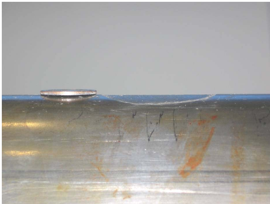
Figure 5.15: Side view of accelerated corrosion, 20% through thickness
