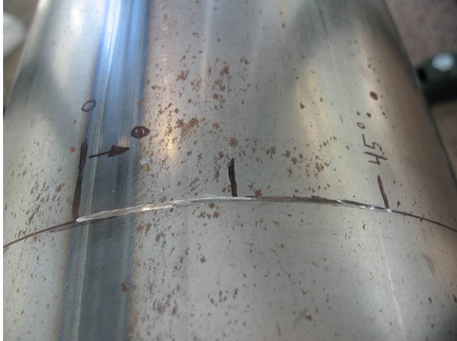
Figure 5.2: Circumferential notch, 50% through thickness, 0.0^\circ to 45.0^\circ
