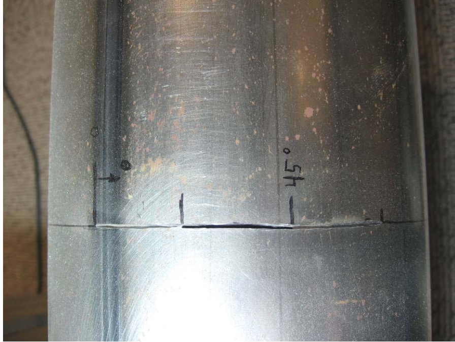
Figure 5.5: Circumferential notch, 100% through thickness, 22.5° to 45.0°
