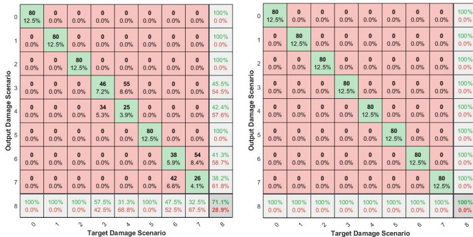
Figure 6: Confusion matrices obtained by SAE. On the left for 15 hidden layer neurons. On the right for 25 hidden layer neurons
