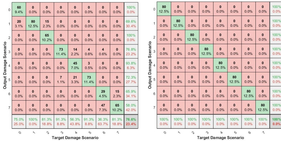
Figure 7: Confusion matrices obtained by CNN. On the left for 250 elements to construct the pooling layer. On the right 100 elements to construct the pooling layer
