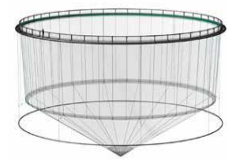
140m circumference cage (adapted for 30 m depth)
