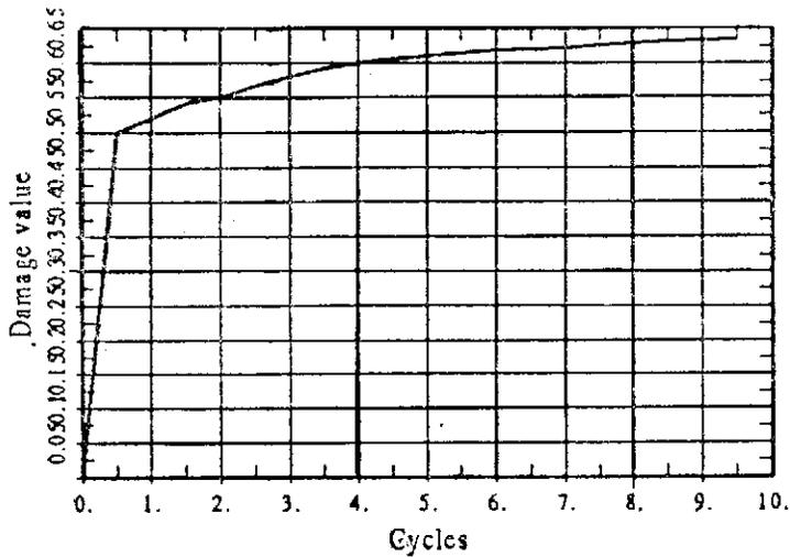
Fig. 4. — Damage evolution of a beam midpoint in a fatigue test.
