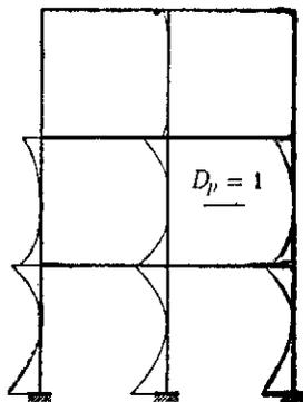
Fig. 10. — Distribution of sectional damage  $D_p$ , after mild earthquake.
