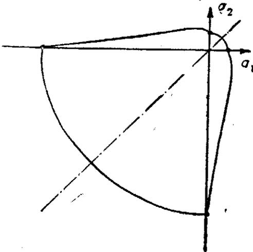
Fig. 2. — Damage Yield in the principal plane  $\sigma_1 - \sigma_2$ .
