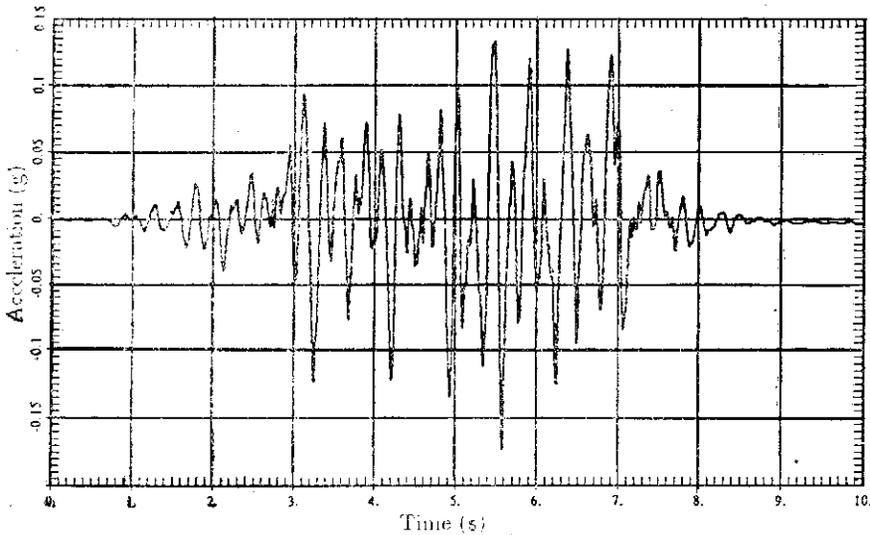
Fig. 6. — Synthetic accelerogram.
