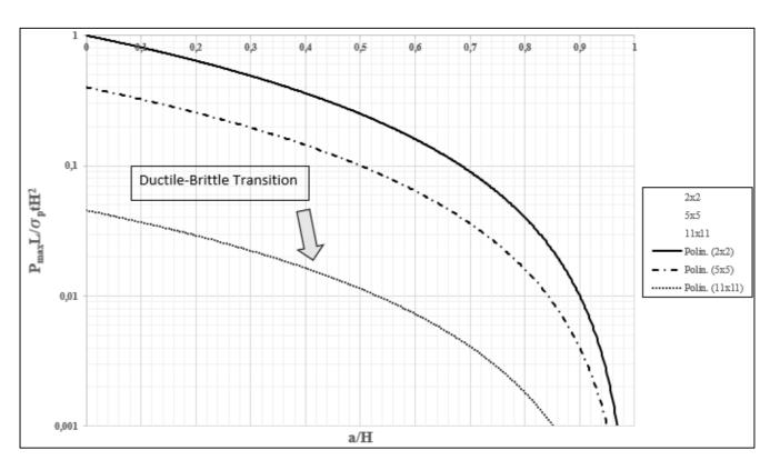
• This behavior mirrors material fracture, where a crack becomes critical and leads to sudden failure after reaching a certain length.
