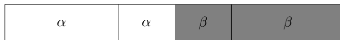
Figure 5: One mixed cell ( f^\alpha = f^\beta = \frac{1}{2} ) surrounded by two pure cells. Between the left and middle cells, the face volume fractions are: f_+^\alpha = \frac{1}{2} (constant) and f_+^\alpha = \frac{1}{4} (linear).
