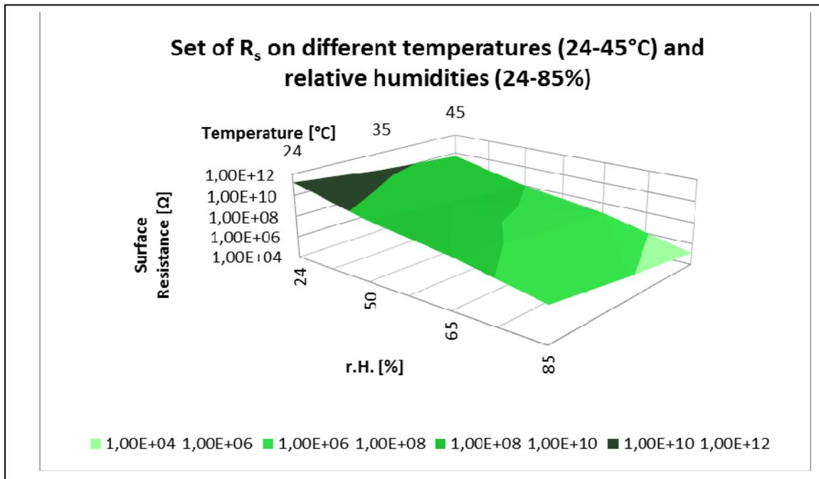
Figure 10: Set of  $R_s$  on different temperatures and relative humidities
