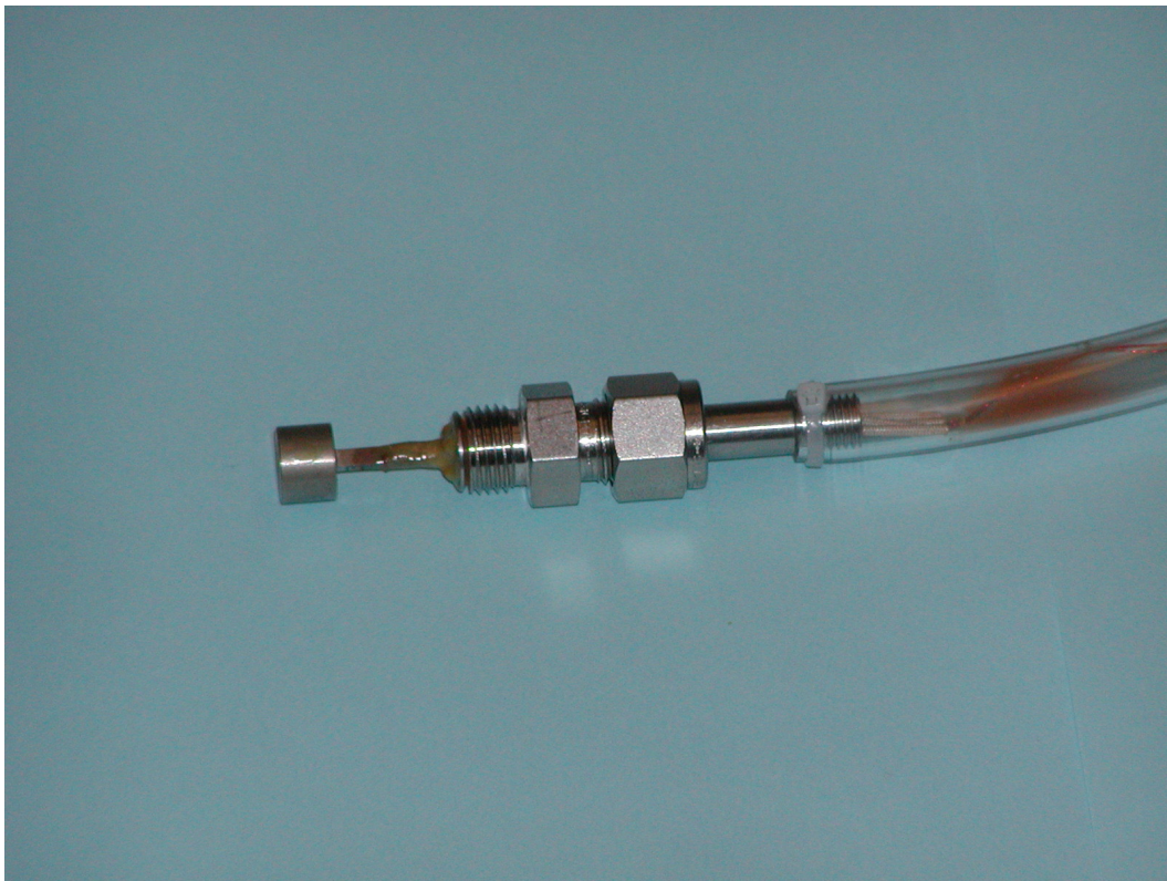
Figure 3-4. Photograph of a Completed Surge Detection Probe Ready for Installation in the Laboratory Compressor.
