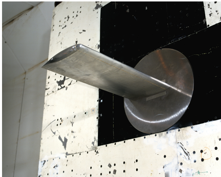
Figure 1: Benchmark SuperCritical Wing (BSCW) with splitter plate. [13]
