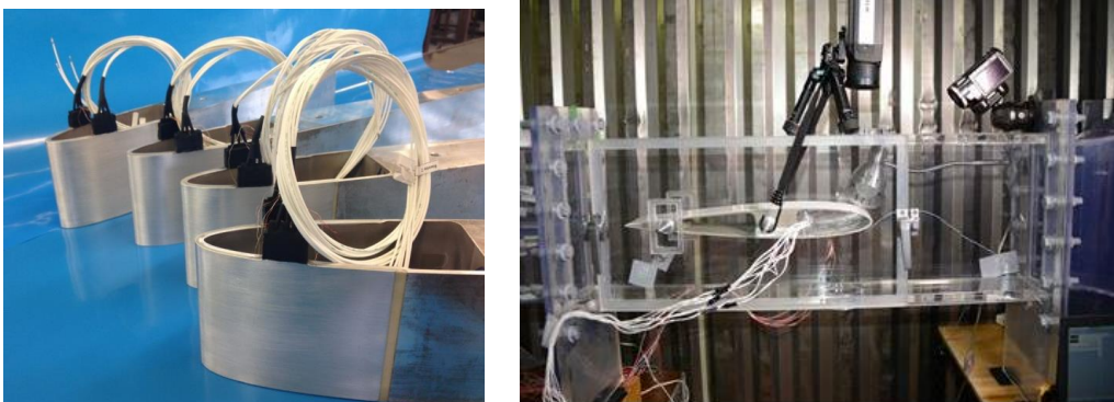
Figure 6 : airfoil mock-up equipped with electrothermal mats and icephobic coatings in icing wind tunnel.
