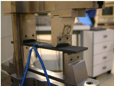
Figure 10 : experimental and simulation results of composite bending test
