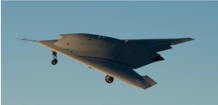
Figure 13 : Neuron low observability demonstrator
