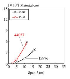
Figure 7: Material cost of simple supported beam versus span
