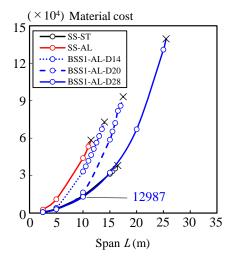
Figure 8: Material cost of BSSs with a strut versus span
