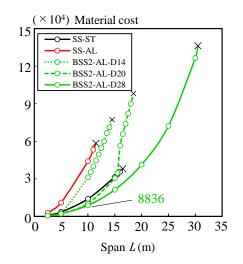
Figure 9: Material cost of BSSs with two struts versus span
