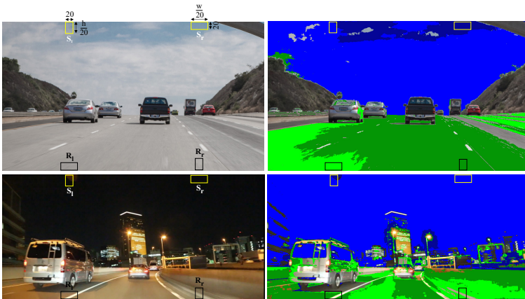
Fig. 2. Dynamic averaging for ground and sky region under day or night conditions
