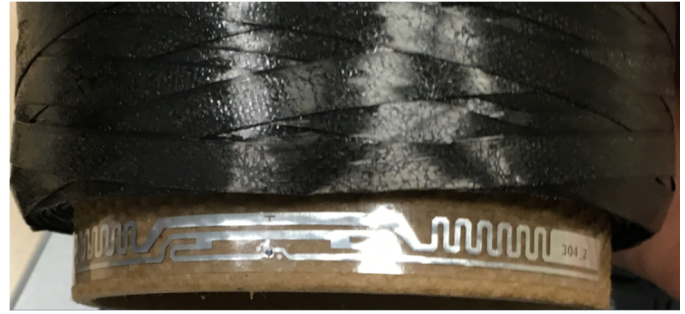
Figura 4. Examples of RFID stickers used to track and validate by-products before being reused.
