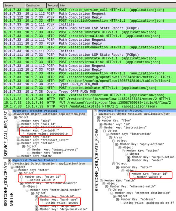
Fig. 3: Multilayer E2E TE-aware service orchestration Wireshark capture.
