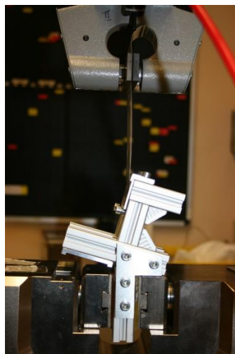
Fig. 4: Lower holding device in clamp with foil exit angle of 15°
