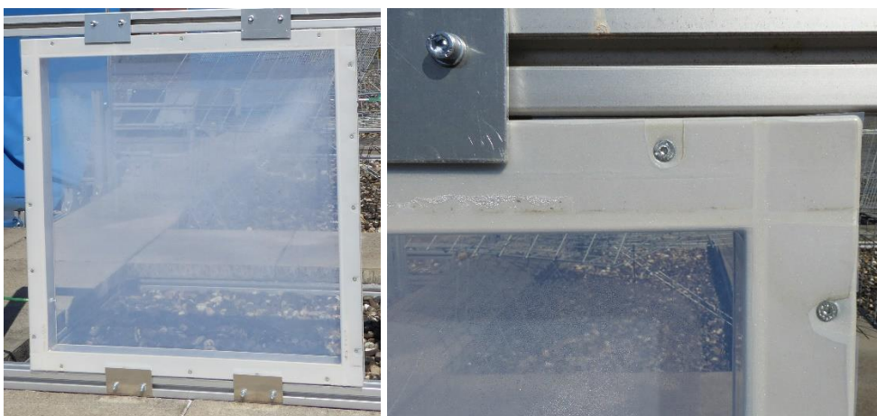
Fig. 9: welded ETFE demonstrator and detail of the seam
