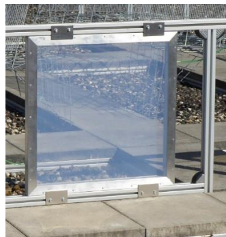
Fig. 7: outdoor installation of ETFE cushion bonded by adhesive
